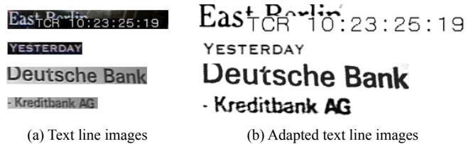
Figure 8. Example resulting images of dynamic contrast/brightness adaption. Contrary to the originals, the revised images are suitable for being processed by OCR engines, as the background has been removed.
